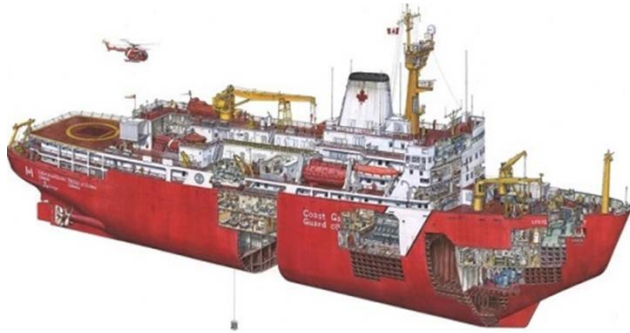
Figure 2-2 Cross-Section of an Icebreaker (Louis St. Laurent)
